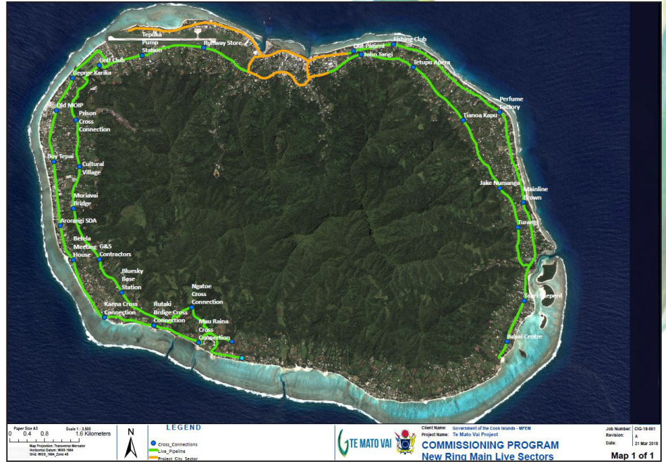
Aerial plan showing progress of the ring main commissioning works
