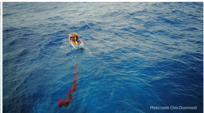
Dye plumes used to measure currents and water mixing off the coast of Rarotonga. Photos from UNSW.
