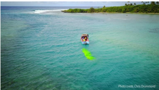
Dye plumes used to measure currents and water mixing off the coast of Rarotonga. Photos from UNSW.
