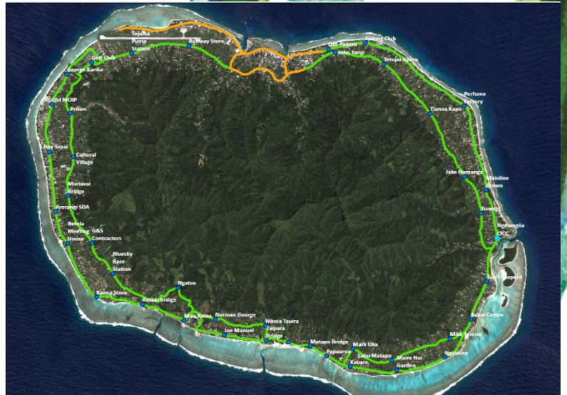
Aerial plan showing the living of all new ring mains (as at 18 May 2018)
